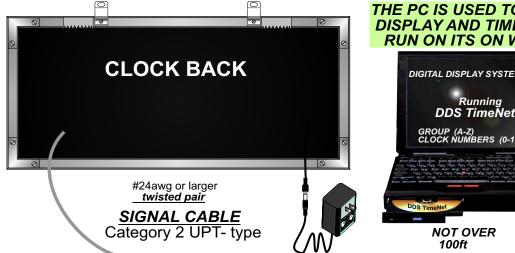
THE PC IS USED TO SET THE LOCATION DISPLAY AND TIME. THE CLOCK CAN RUN ON ITS ON WITHOUT THE PC.
