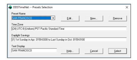
To use a preset, select it from the "Preset Name" dropdown list, and press the "Select" button. The Time Zone, Daylight Savings and Text Display are inserted into the selections for the current group in the main dialog window. This is simply a fast way to enter group selections for commonly used combinations.
