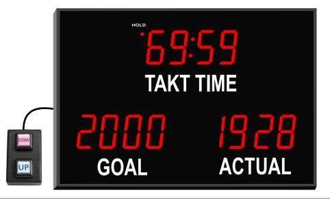
**TAKT**: COUNTS DOWN FROM SET START TIME. AT ZERO, RESETS TO START AND COUNTS DOWN AGAIN **GOAL**: AUTOMATICALLY INCREASES WHEN TAKT TIME = 0 **ACTUAL**: MANUAL COUNT UP VIA UP/DOWN SWITCHBOX OR VIA DRY CONTACT(OPTIONAL)
